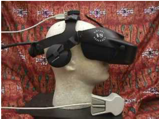
Figure 2: Virtual Research V8 Head Mounted Display and 3DOF mouse
