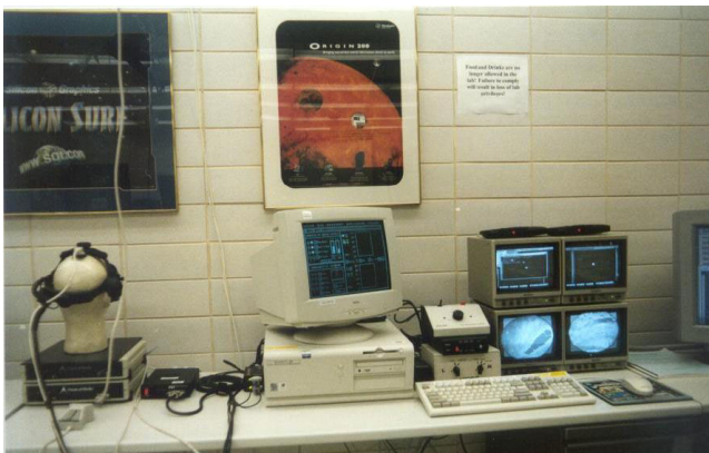
Figure 3: Eye tracking Control Computer with left and right eye video screens
