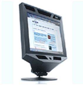
Figure 1. Tobii ET-1750 binocular eye tracker.
