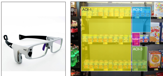
Figure 8: Tobii Eye Tracking Glasses and AOI Distribution
