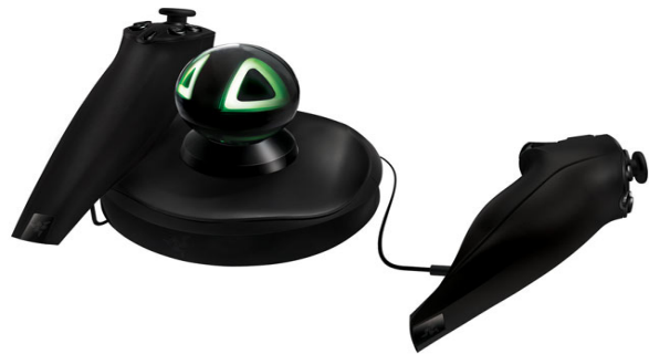
Figure 2. The Razer Hydra used to manipulate objects in the virtual task.
