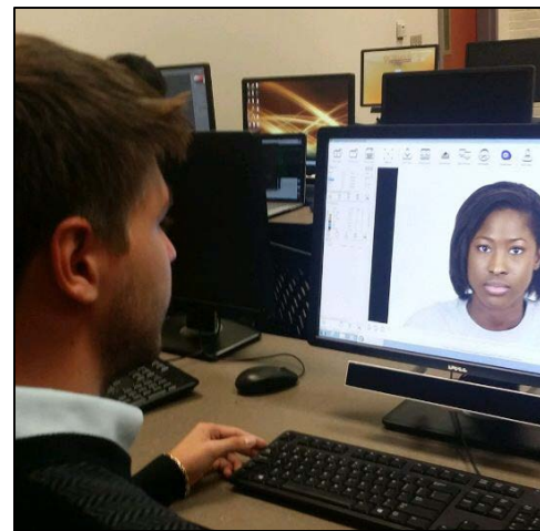
Figure 1: A behind the shoulder picture of the experimental set up. The Gazepoint Eye Tracker is mounted below the monitor shown in the picture. A participant is viewing an image in the Gazepoint Analysis software.
