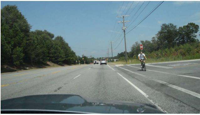
Figure 3. An example miss (automation fails to detect a bicyclist that is present)
