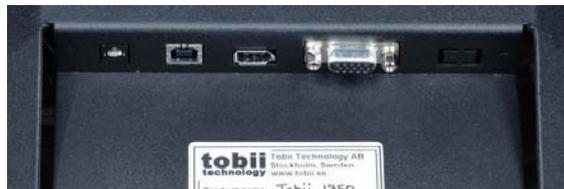
**Figure 2: On the backside of the Tobii 1750 four cables are connected, from left to right power, USB, Firewire and monitor cables**
