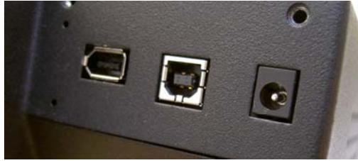
**Figure 3: The cable connections on the Tobii x50. From left to right, Firewire, USB and power.**
