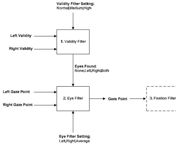
**Figure 27: Chart describing how the validity and eye filters provide data to the fixation filter.**
