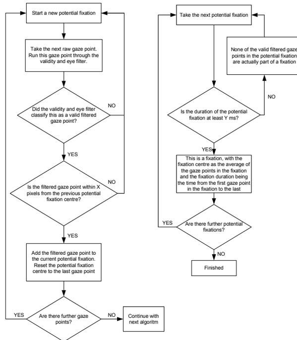
**Figure 28: The fixation filter algorithm**
