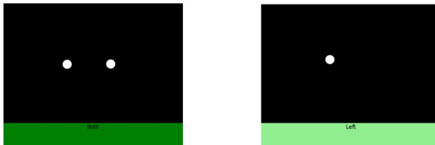
**Figure 15: The track status meter to the left shows perfect tracking while the one to the right indicates that only the left eye of the user can be found.**
