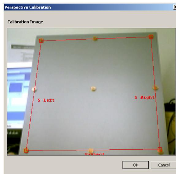
**Figure 13: Perspective calibration is a crucial part of the Scene stimulus setup**
