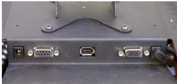
**Figure 4: On the back side of the Tobii ET 17 four cables are connected, from left to right, power, serial, Fire wire and monitor cables**
