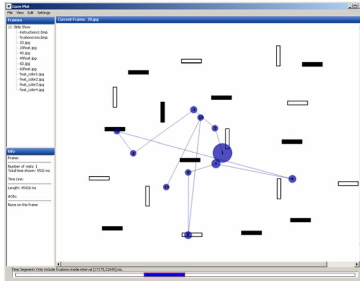
**Figure 20: The Gaze plot visualizes the scan path of a user**
