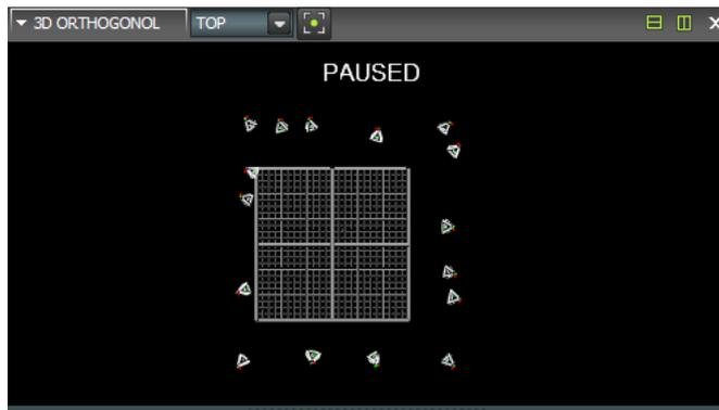
**Camera**      Raw 2D motion capture data from an individual Vicon camera.
