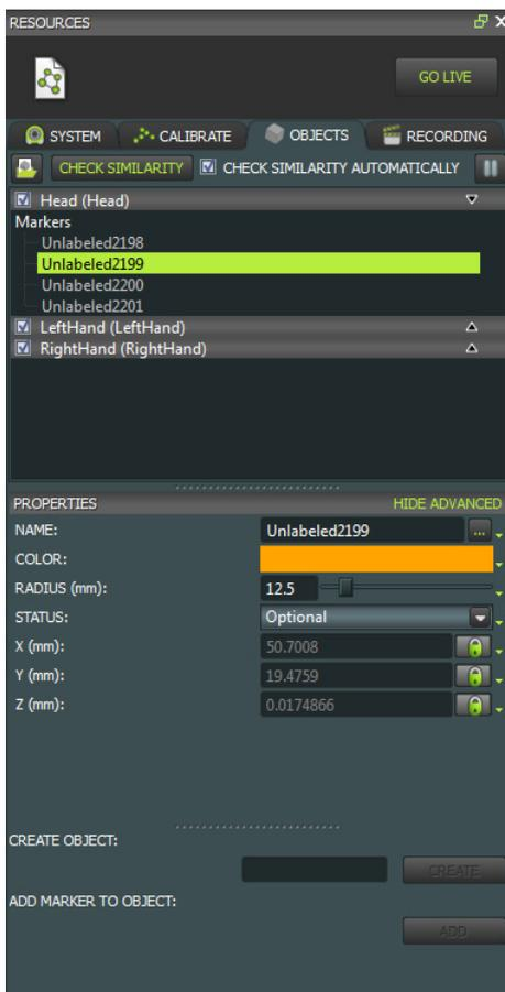
Prepare and manage the objects whose motion data you want to track in Vicon Tracker on the Objects tab in the Resources pane. Objects are a rigid, asymmetrical arrangement of at least three markers. Multiple objects can be defined to track many rigid bodies at the same time.
