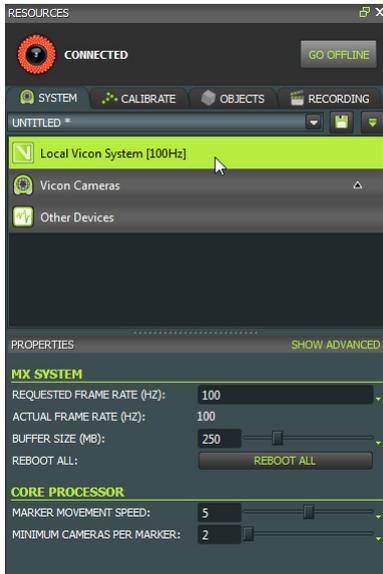
The Local Vicon System node enables you to configure the Vicon system capture rate and the amount of memory allocated to Tracker for motion capture, manage the way Tracker is to produce real-time 3D representations of the objects whose motion is being captured, and specify the identification and connection settings for the Tracker host PC.
