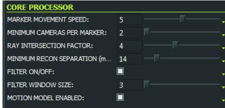
The Core Processor receives data from the Vicon cameras and transforms the data to the trajectories or segments that your MX system is tracking.
