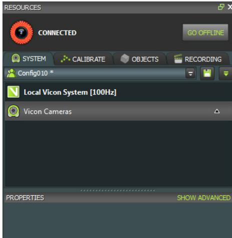
You manage the system components, calibration, objects, and recordings/playback of your Tracker system in the Resources pane.
