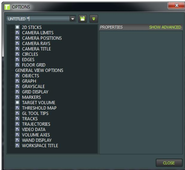
You access this dialog box from the **Window** menu or by pressing F7. You can save the settings that you make in this dialog box, which enables you to customize sets of options to use for different types of motion capture projects.
