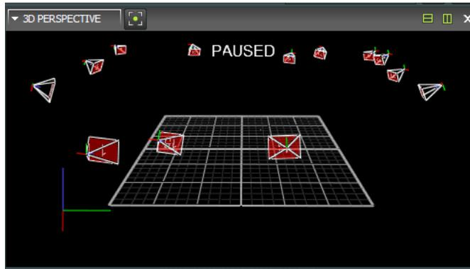
**3D Orthogonal**      Motion capture data in 3D viewed from a specified point of sight or direction of the capture volume.
