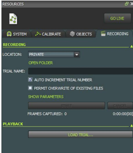
Save and play back recordings of trial data, using the controls on the Recording tab in the Resources pane.
