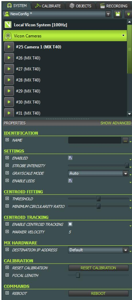
You manage the identification and configuration settings for each Vicon camera connected to your Vicon system with the **Vicon Cameras** node.
