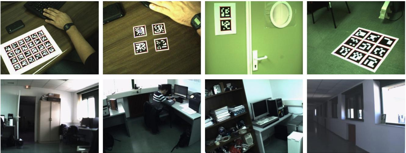
**Fig. 11.** Image examples from video sequences used to test the proposed fiducial marker system. First row shows cases of correct marker detection. Second row shows cases where false positives have not been detected.
