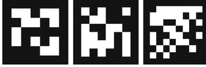
Fig. 3. Examples of markers of different sizes,  $n$ , generated with the proposed method. From left to right:  $n=5$ ,  $n=6$  and  $n=8$ .
