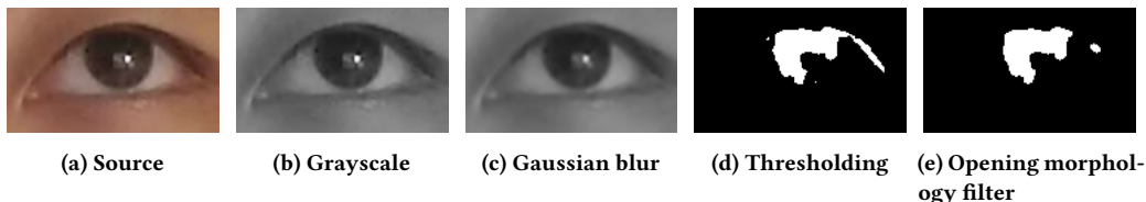
Figure 1: Image preprocessing pipeline to isolate the pupil region.
