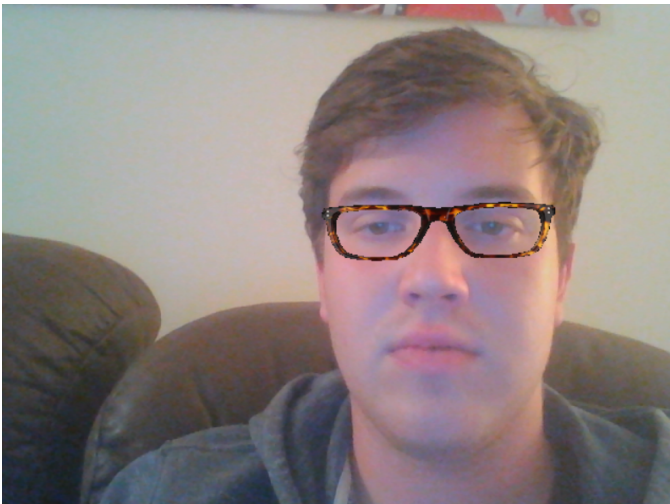
Figure 7: Dlib detection and glasses drawn with no facial rotation
