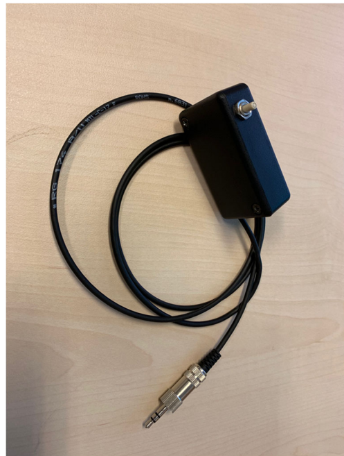
Fig. 6 Button box for Tobii Pro Glasses 2. As long as the button is pressed, this box sends a TTL signal over a 3.5 mm jack that can be plugged directly into the sync port on the Tobii Pro Glasses 2 recording unit
