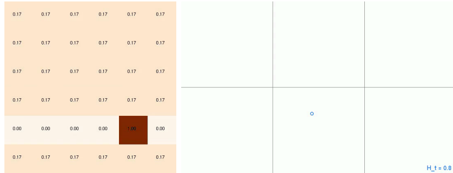
(b) Near maximum entropy, H_t = 0.8 , since most transitions are equally likely although gaze is largely confined to a single AOI. In this case entropy should be 0.
