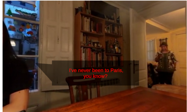
Figure 4: The Speech-Bubble method uses triangular "tails" to point a user towards the speaker.
