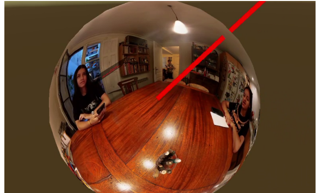
Figure 2: Videos are decompressed to a texture and applied to a sphere with inverted normals and backface culling. This setup allows for better third-person viewing for researchers outside the head-mounted display with a minimal performance impact. The red line is only rendered in third-person views and represents the user's gaze vector.
