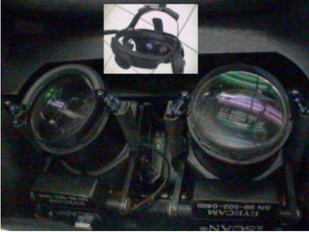
Figure 2. Binocular eye tracker optics (with HMD inset above).
