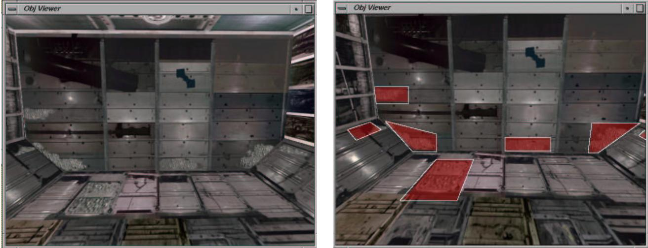
Figure 14. Registering ROIs in VR: (a, left) simulated corrosion; (b, right) highlighted environmental defects.
