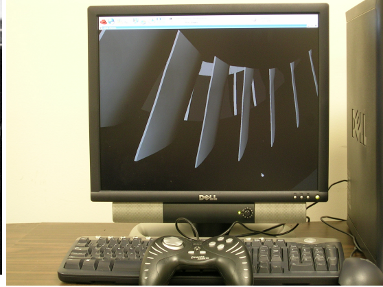
Figure 3.4: Visual output from the virtual borescope and user controls via the gamepad.
