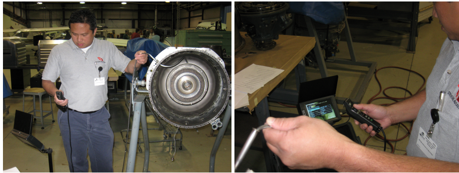
Figure 8.1: Inspection of PT-6 aircraft engine using borescope (left) and operator view of the camera output on the screen (right).
