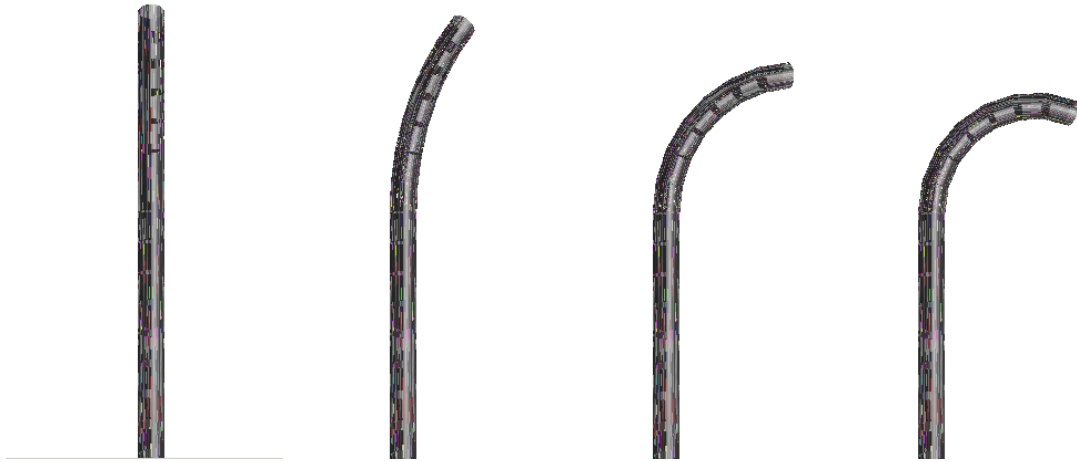
Figure 6.1: Visualization of the virtual borescope's articulation. This view is never seen by the user, instead, the user's viewpoint is from the probe's tip.
