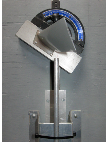
Figure 7.4: Top-view of apparatus designed to simulate feed and interaction of borescope probe with engine blade.
