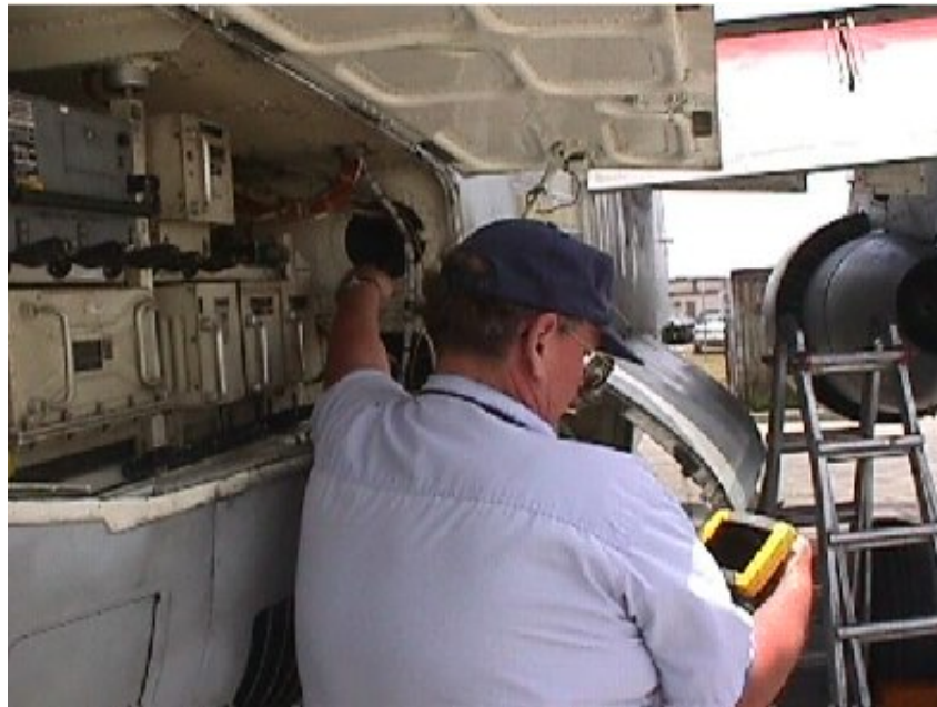
Figure 2.6: Inspection of aircraft components using the video borescope.
