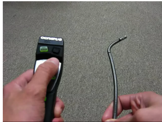
Figure 2.3: Articulation of borescope tip.
