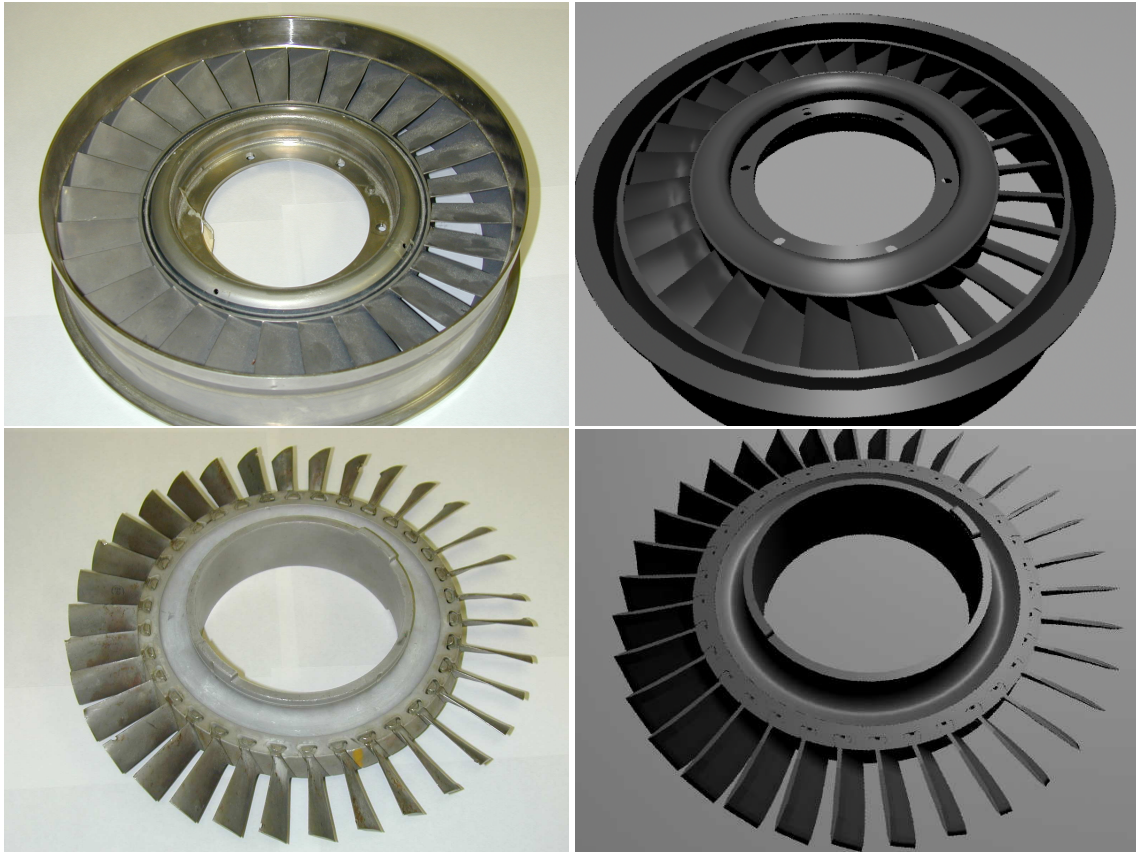
Figure 3.1: Actual and modeled engine sections (left, right) of stator (top) and rotor blades (bottom).
