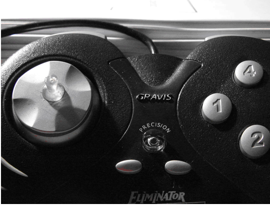
Figure 3.3: Orientation and translation control of the virtual camera with the directional pad and buttons (1 and 4) on the gamepad.
