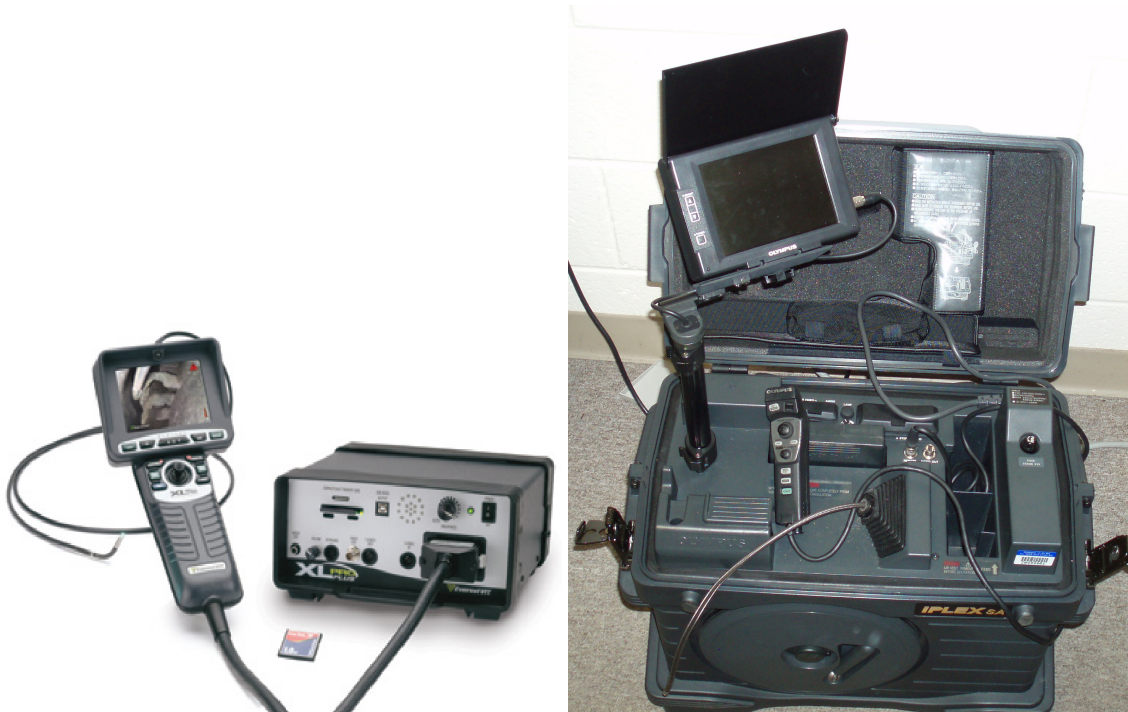
Figure 2.1: Two different types of video borescopes: XL PRO™Plus VideoProbe from Everest, and The IPLEX Borescope from Olympus.
