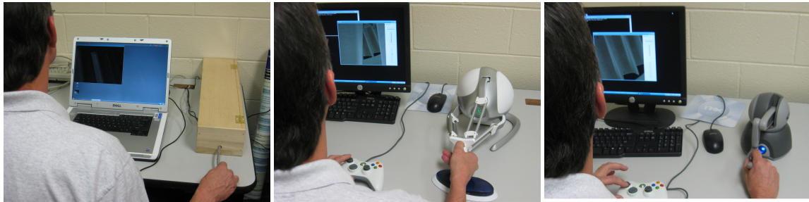
Figure 6.7: Operational evaluation of (from left to right) the Haptic box, Falcon and Phantom Omni interfaces with the borescope simulator.
