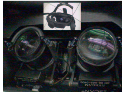
Figure 3: Binocular eye tracker optics (w/HMD inset).
