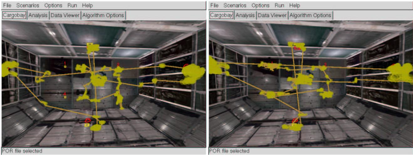
Figure 10: Detected fixations (2-tap vel. filter, ungrouped) prior to (a, left), and following (b, right) binocular scale factor adjustment.
