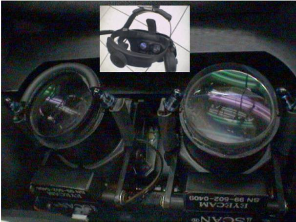
Figure 2: Binocular eye tracker optics (w/HMD inset).
