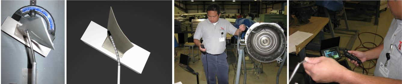
Figure 1: Visual comparison of intersection response of actual and virtual probe at 30° angle of incidence (for visualization purposes only—the user's viewpoint is from the probe's tip); inspection of PT-6 aircraft engine using actual borescope, with operator's view of the camera output.
