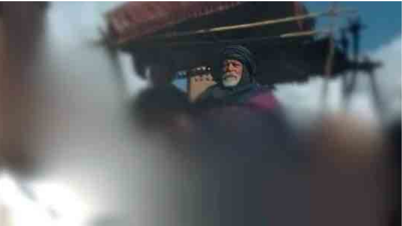
Figure 1. Gaze-contingent display shows a scene from the movie The Gladiator . As the user focuses on the face of the shot's main character, all other display content is rendered at reduced resolution. This type of display can be used for gaze-contingent compression purposes or for the study of human visual perception—in this case the display is used to study glaucoma patients. (Original image © 2000 DreamWorks SKG and Universal Studios; gaze-contingent rendering and resolution map courtesy of Bill Geisler and Jeff Perry.)
