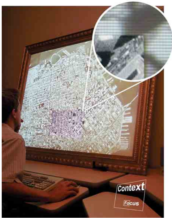
Figure 2. Focus plus context screens complement a monitor-sized high-resolution area in the screen center with a large low-resolution space in the periphery. Courtesy of the Palo Alto Research Center.
