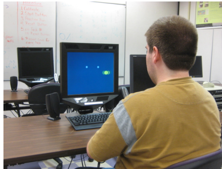
Figure 5: Example of participant at eye tracker during calibration. During calibration, a yellow dot moves to nine fixation targets while two grey dots display the participant's eyes in the camera's reference frame (as an indication of their relative position to the camera).
